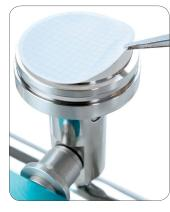
2. Filter support can be easily removed
